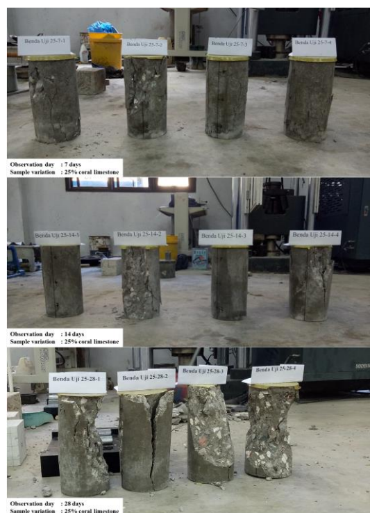
Figure 9. Fracture pattern of 25% coral limestone variation sample.
