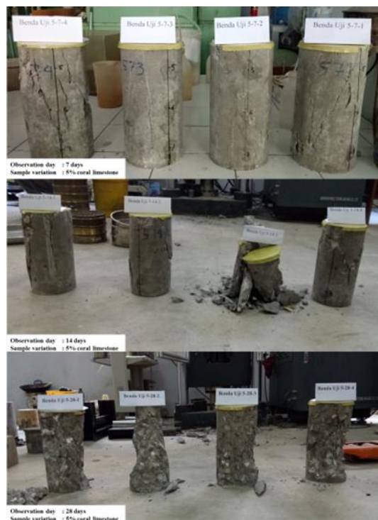
Figure 8. Fracture pattern of 5% coral limestone variation sample.
