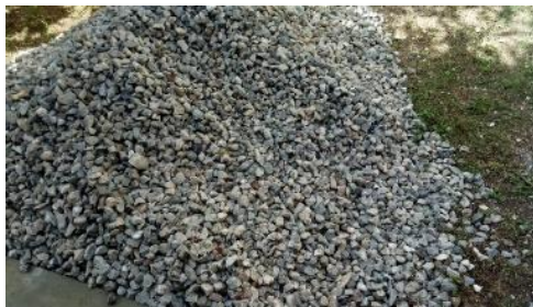
Figure 3. coarse aggregate (maximum size of 20-30 mm).
