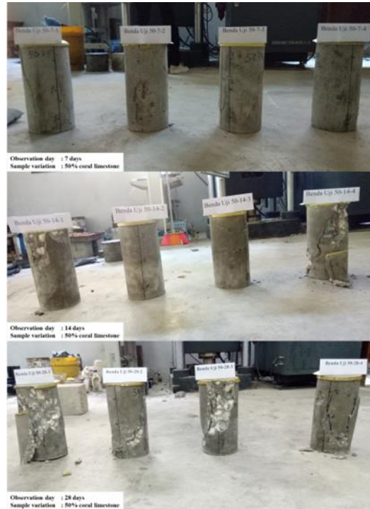
Figure 10. Fracture pattern of 50% coral limestone variation sample.
