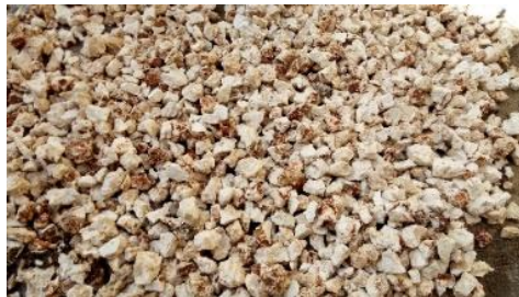
Figure 4. coral limestone maximum size 40 mm.
